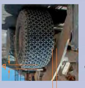
dirt build-up are taken forces and possible CHAINS, centrifugal fit tyre protection clearances required to These are the minimun
